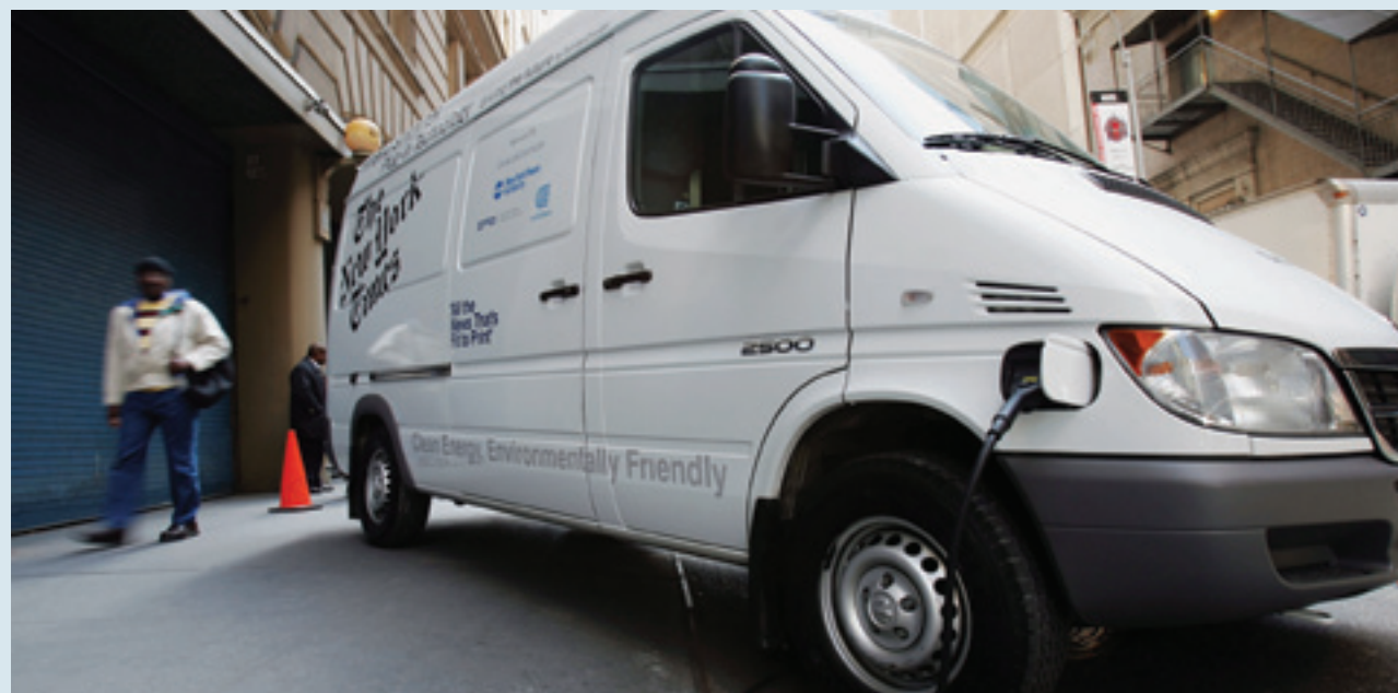
A New York Times Dodge Sprinter plug-in hybrid electric vehicle (PHEV), which will be used for newspaper delivery, is seen April 11, 2007 in New York City. The vehicle is the first medium-duty plug-in hybrid vehicle on the East Coast and can operate up to 20 miles in zero-emission electric mode or as a hybrid with a diesel.
