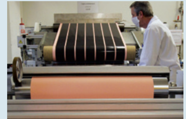
A worker checks production of lithium-ion automotive batteries in a Johnson Controls Advanced Power Solutions plant.
